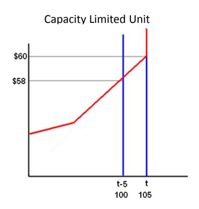
105 megawatt capacity 5 megawatt ramp rate
