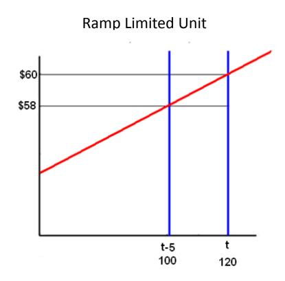
200 megawatt capacity 30 megawatt ramp rate
